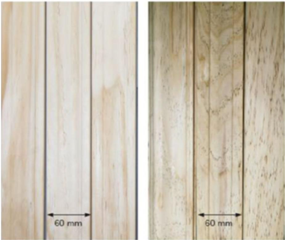
**Fig. 1** Low (left) and prevalent (right) resin canals features (dark spots) in appearance grade radiata pine. Photo credit: SWI (Solid Wood Initiative), New Zealand
