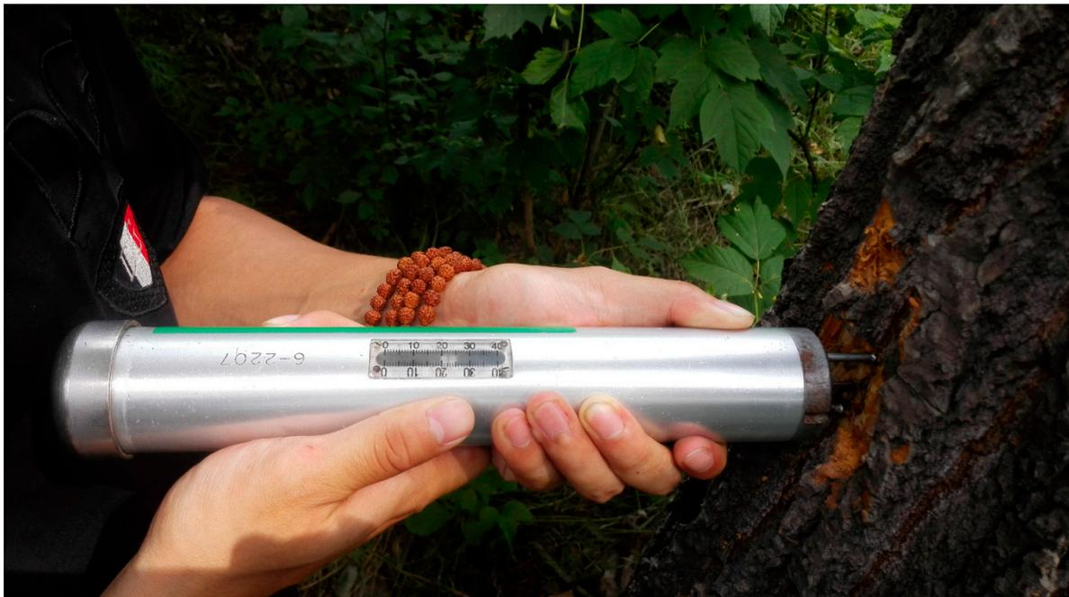
**Figure 3.** The Pilodyn wood tester (photo credit: Shan Gao).
