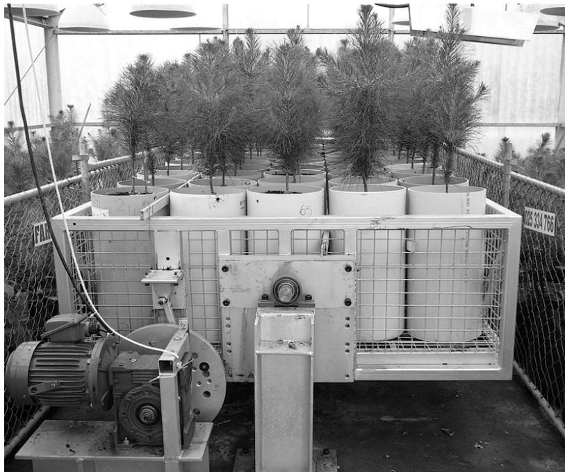
*Figure 1: Rocking machine simulates the movement of trees under wind of 10 km h<sup>-1</sup>.*
