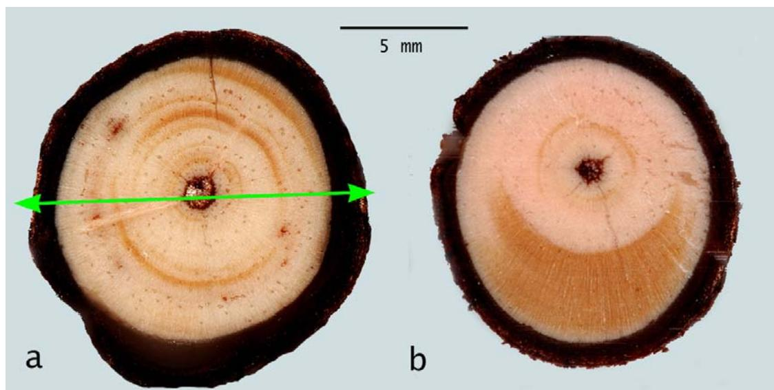
Figure 4: stem cross-sections for rocking tree showing compression wood in thin arcs at random (a) and leaning tree showing a continuous wedge of compression wood on the underside of the stem (b). The green line shows the direction of rocking.
