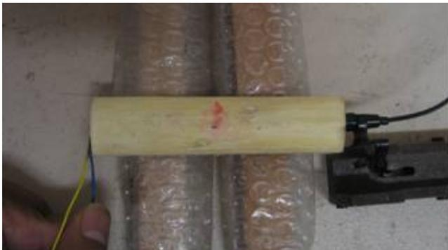
Resonance occurs at higher frequencies in small samples, output is captured by microphone and processed.
